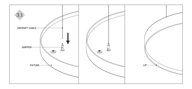
$3A.1 \qquad \text{From the top of the fixture, insert each aircraft cable into the gripper until the desired height is achieved.}$
