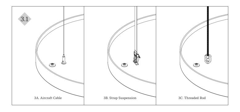
3.1 To properly install the fixture reference 3A, 3B or 3C to complete the installation depending on the suspension type.
