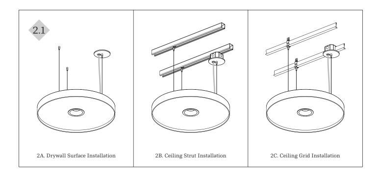
$2\textbf{.}1 \\ \text{To properly install the fixture reference 2A, 2B or 2C to complete the installation depending on the surface type.}$
