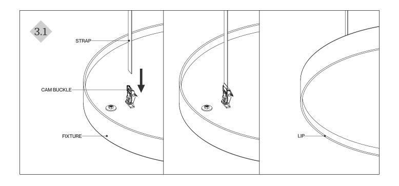
$3B \hbox{.} 1 \qquad \text{From the top of the fixture, insert each strap into the cam buckle until the desired height is achieved.} \\$
