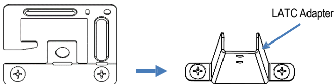
FIG. 12: SWAPPING T-GRID CLIP FOR LATC ADAPTER
