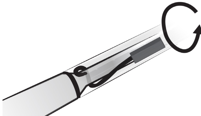
Fig. 8-7: Twist the Solar Module Cables around the Pole to Provide Strain Relief
