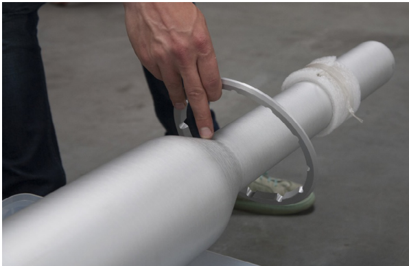
Fig. 8-2: Orient Bottom Adapter Ring with Bumpers Facing Top of Pole
