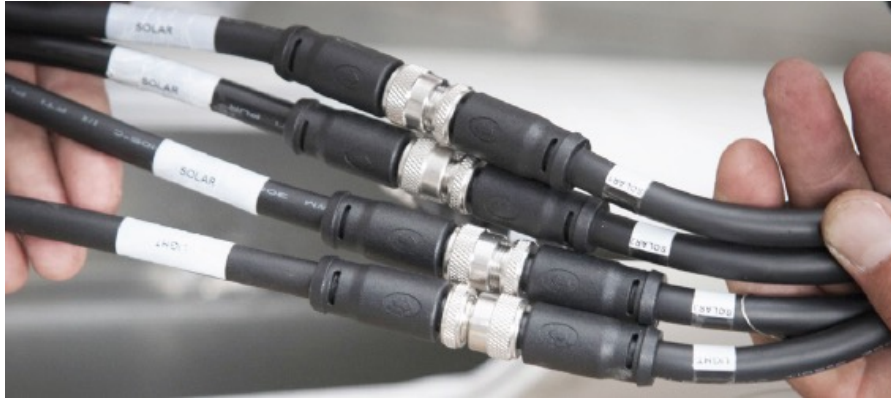
Fig. 12.1-6: Breakout Cable Connectors to Solar and Light Cables
