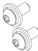
Fig. 2-12: 1/4-20 x 5/8 Button Head Screws with Lock and Flat Washers for Control Unit Mounting
