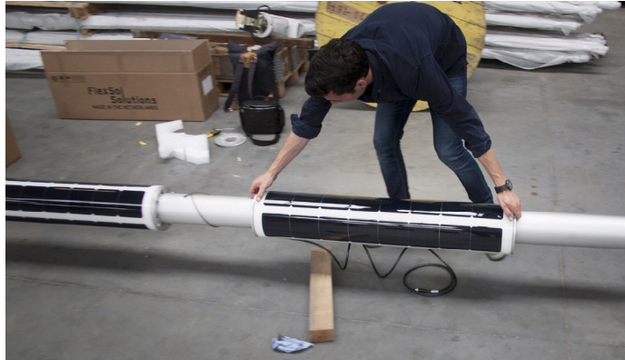
Fig. 9-2: Slide Intermediate Solar Module over Pole
