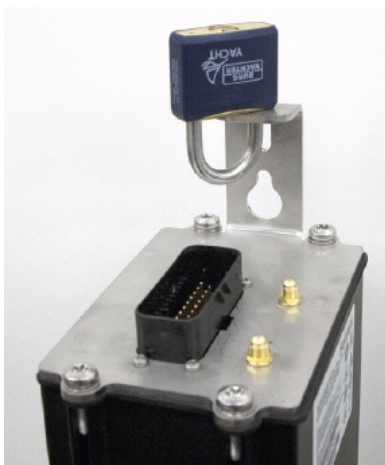
Fig. 12.1-9: Installing a Lock on the Control Unit
