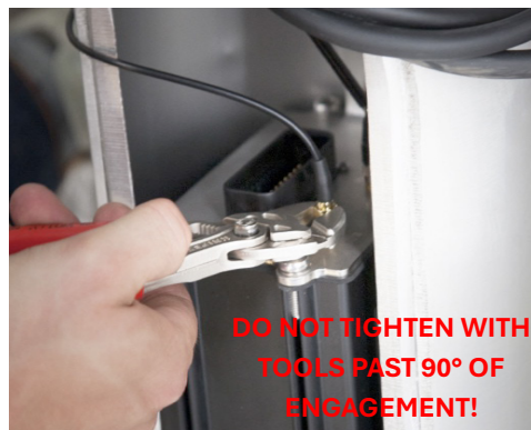
Fig. 13-2: Tighten Antenna Connections with Tools up to 90°
