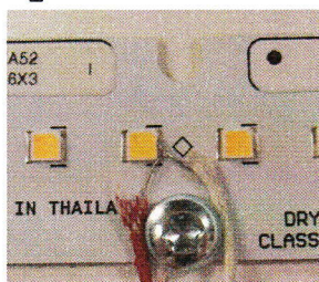
LED Typical-Thermocouples mounted Per manufacturer LM80 Data
