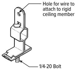
**STEP 3:** Depending on the placement of the fixture, it may be necessary to drill holes in the back-side of the fixture to match up to the GAT fasteners.
