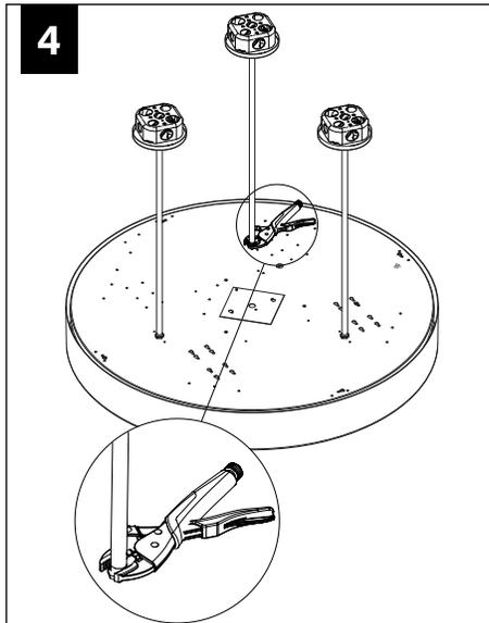
1. ATTACH THE STEM TO COVER. DO NOT OVER TIGHTEN STEM, THIS MAY CAUSE PINCHED WIRES.
