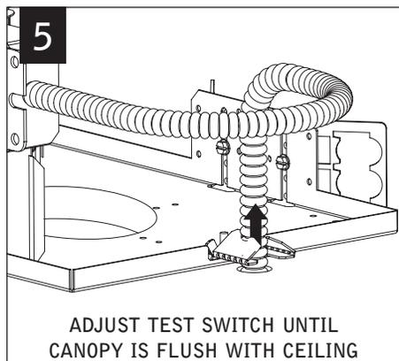
ADJUST TEST SWITCH UNTIL CANOPY IS FLUSH WITH CEILING
