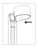
Insert the device body and lock using Torx T9 key for upper screws and Allen key size 2.5mm for lower screws
