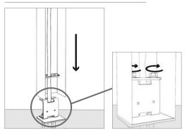
Insert the device body on the bracket and lock the bolts using a CH5 10Nm key
