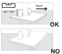
Check that everything is perpendicular to the bubble level of the surface, an incorrect positio-ning will cause the device to become unstable
