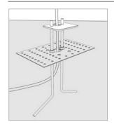
Cement the anchor bolt flush by passing the cable through the appropriate openings
