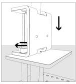
Insert the bracket and lock the bolts with a CH10 10Nm key
