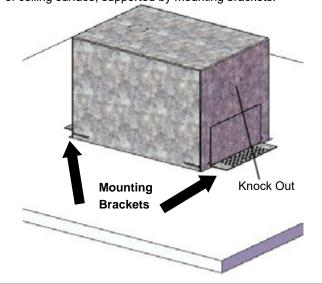
3. Loosen all four wingnuts slightly and position the housing so that is it recessed in the opening by about 1/4". Tighten all wingnuts.
