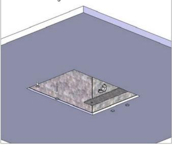
4. Attach the fixture to the face plate as shown. Connect fixture wires to building wires, **RESPECTING POLARITY**. Mount the assembly into the back box. Adjust accordingly so the fixture face is flush with the ceilling surface.
