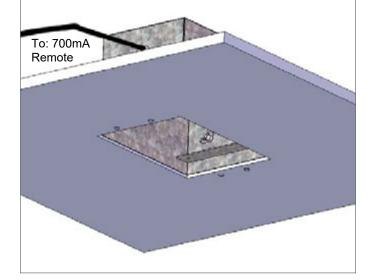
5. Apply fiberglass tape around opening and apply plaster. Sand smooth when dry.
