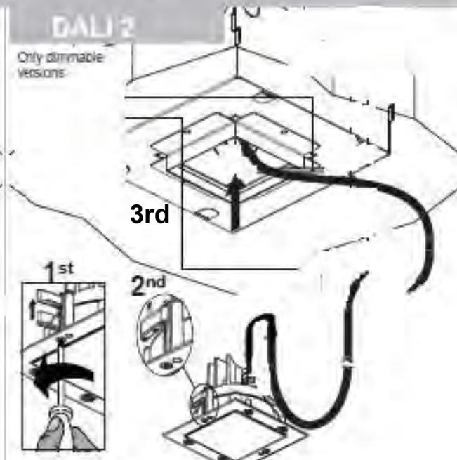
Use a terminal block conforming to EN 60998-2-1 or EN 60998-2-2 with a 3-terminal type, with a nominal voltage of 400V, with a connection capacity of 1.00 to 2.00 mm<sup>2</sup>.
