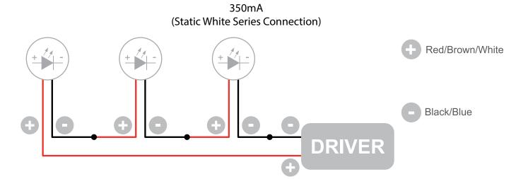
The individual lamps must be connected in series.
