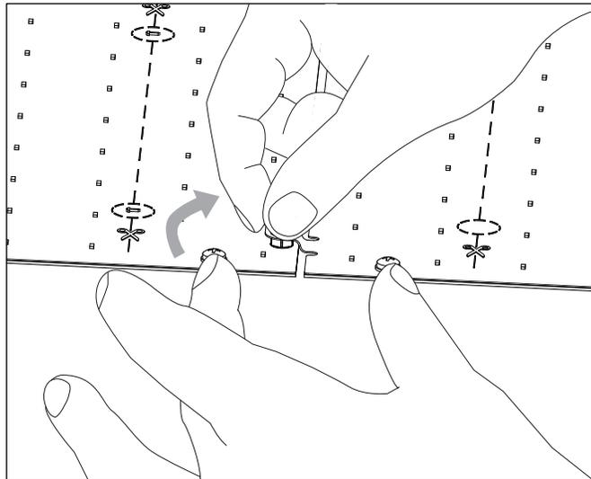
3. Similarly, when disconnecting T-cables from the TILE Interior, the sheet should be restrained while gently separating the connectors.
