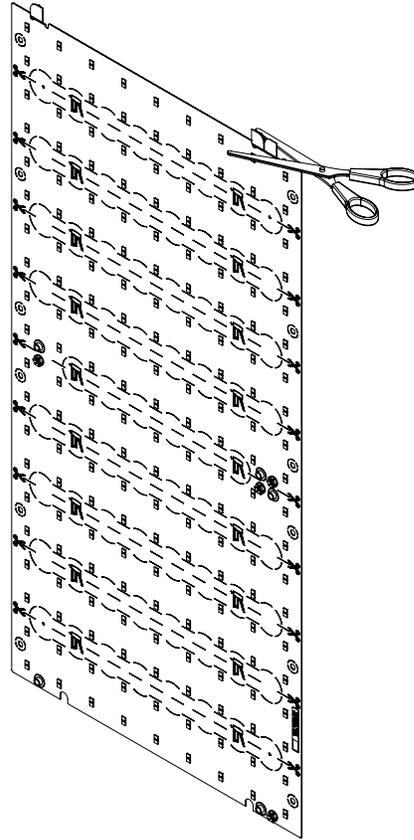
8. Place insulating patches over region of exposed TILE where tabs were cut, as shown.
