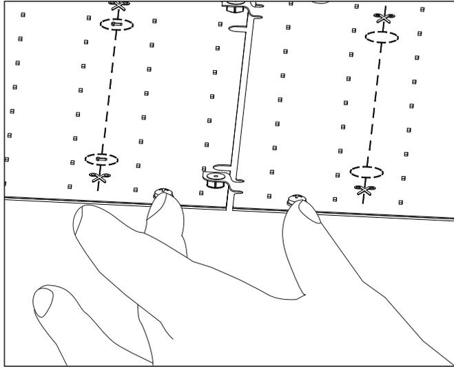
2. Grip the tab between the thumb and index finger. Gently separate the sheets while keeping the sheets restrained.
