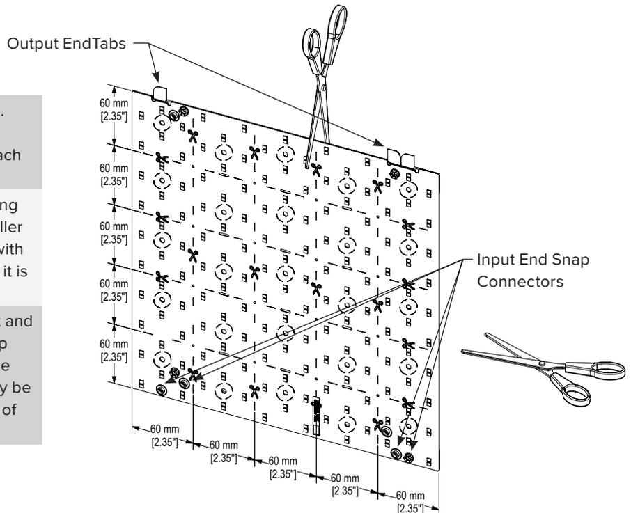
**!** DO NOT CONNECT the T-Cable at the output (tab) end of the Cutout TILE. The T-Cable can only be connected at the input end of the sheet.
