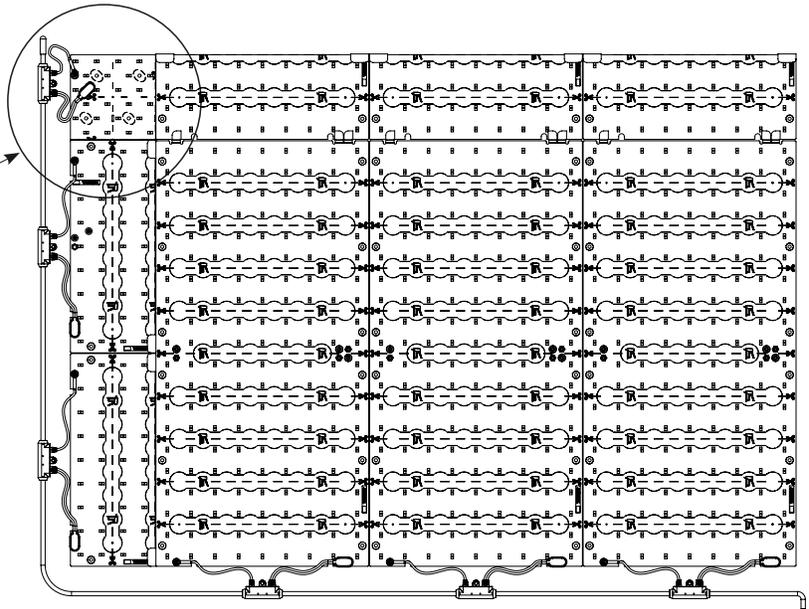
1. Determine the size of TILE Cut-Out required. The sheets are sized to correspond to the allowable cut sizes of the standard sheet (each Cut-Out is 5 x 5 cut increments).
