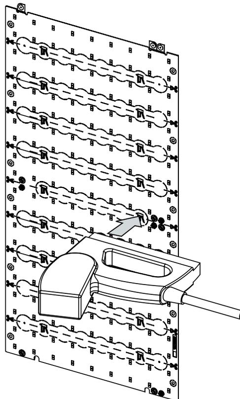
3. Slide the next TILE under the tabs of the first. Ensure that the flexible tabs on the first TILE sit on top of the second.
